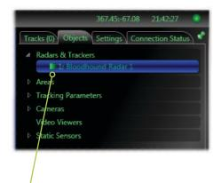
Combined connection and health indicator for a radar and its tracker
